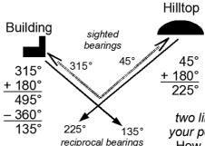
a bearing on a hilltop, 45°, then we add 180° to give 225° - then draw a line from the hilltop on a bearing of 225°. Ideally, where the two lines cross will be
