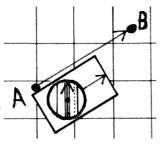
map – with north pointing north on the map! This is a bearing from grid north; if you need to correct for magnetic variation, twist the body to subtract (or add) the magnetic variance from grid north.
